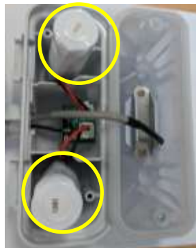
LED POD cover removed. Batteries highlighted
